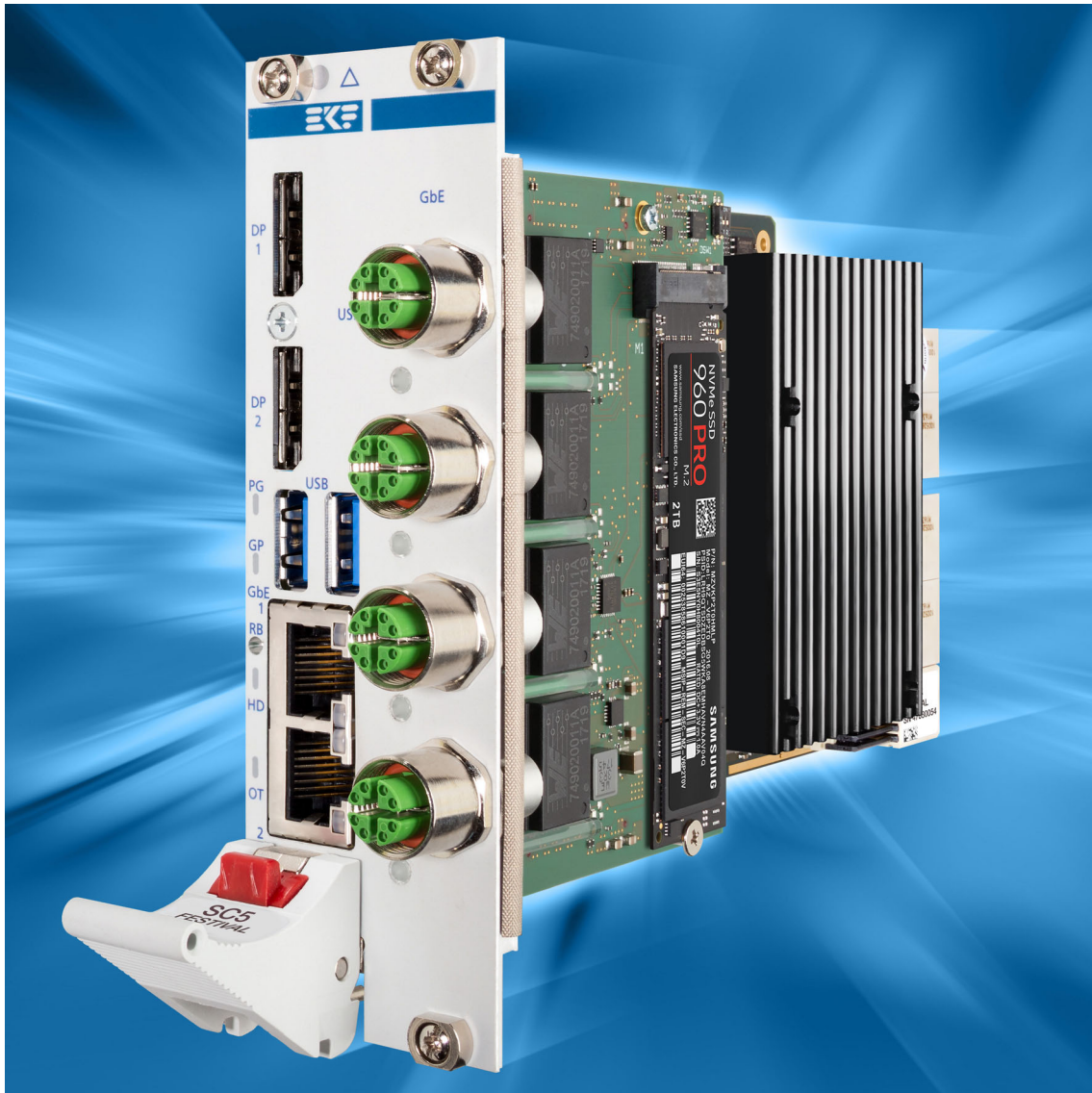
Assembly w. Custom Specific Height CPU Heatsink
